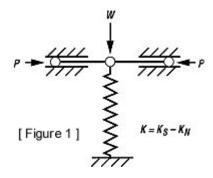
A horizontal-motion isolation system consisting of two beam-column isolators is shown in **Figure 2**. Each isolator behaves like two fixed-free beam columns loaded axially by a weight load W. Without the weight load the beam-columns have horizontal stiffness  $K_S$ . With the weight load the lateral
